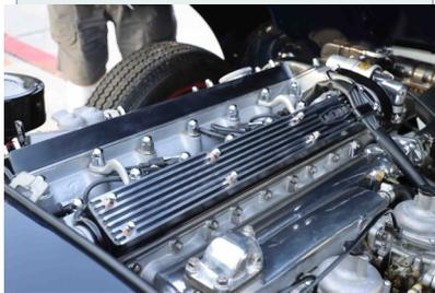
The biggest change between 1961-1967 Series 1 E-Types and the 1968 Series 1.5 was the reduction in the number of carburetors from 3 to just 2 (North America), resulting in a loss in horsepower.
